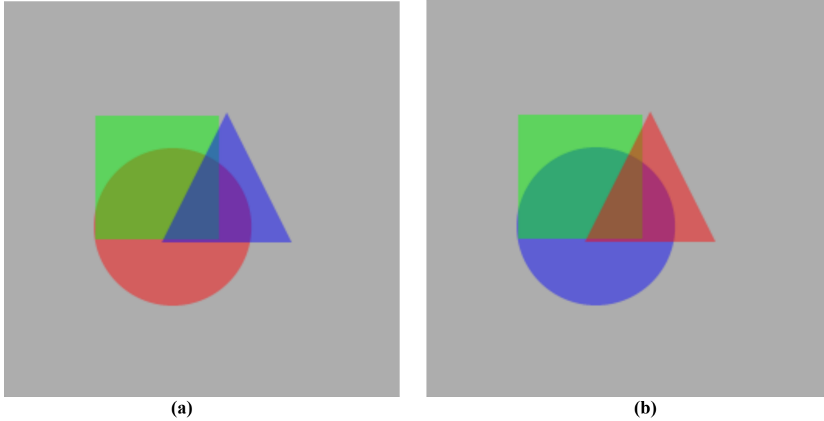
Figure 2.20: The two images illustrate how blending is done in DDS. In both images there are three layers: a circle on the bottom layer, a square on the middle layer, and a triangle on the top layer. In (a) the circle is red, the square is green, and the triangle is blue. In (b) the circle is blue, the square green, and the triangle red. Although each layer has a value of 50% alpha the color of the overlapping areas is different in the two images – this difference is necessary to show the order of the layers, without it it would be impossible to know which shape was on top.
